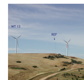
REF mast and WT13 during power curve measuring campaign (North-east view, summer)
